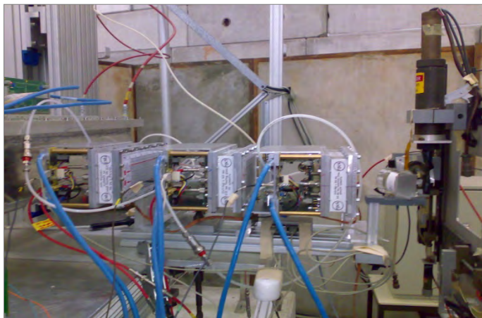
Figure 19.2 In-beam tests of the RPC prototypes
