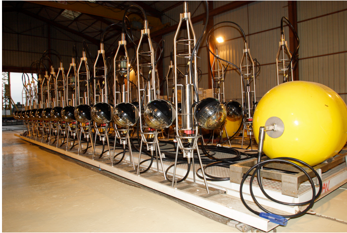
Figure 4.8 A complete ANTARES line prepared for deployment. The 25 storeys, each equipped with 3 optical modules (the shiny spheres) and an electronics container are visible. The large yellow object in the right is the buoy ensuring the line stability under water.
